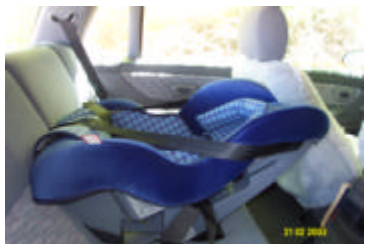
Upper tether attached to seatbelt
