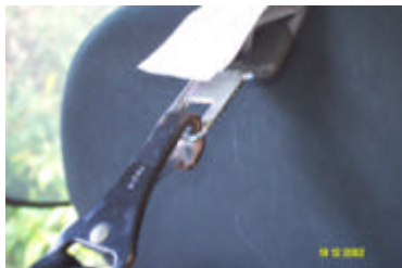
Upper tether attached to seatbelt
