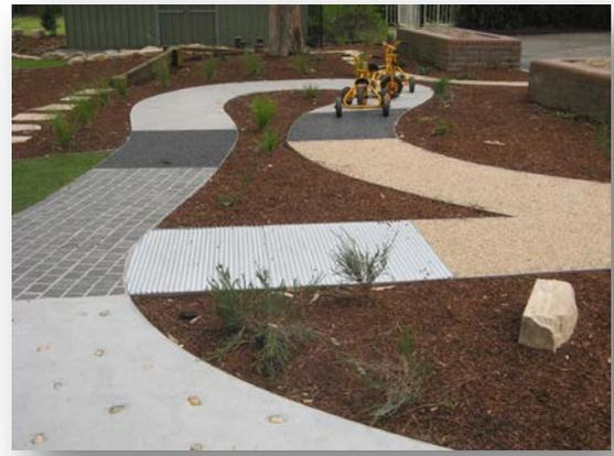
Bike tracks require a hard surfaced path for good traction, approximately 1200-1500mm wide and graded to allow easy movement along the route. Ideally the track surface should be of variable texture to allow children the opportunity to experience both vibration and sound as they travel along the track. Such sensory play experience is very important and can be invaluable in early childhood settings, particularly where children with special needs are part of the community.
